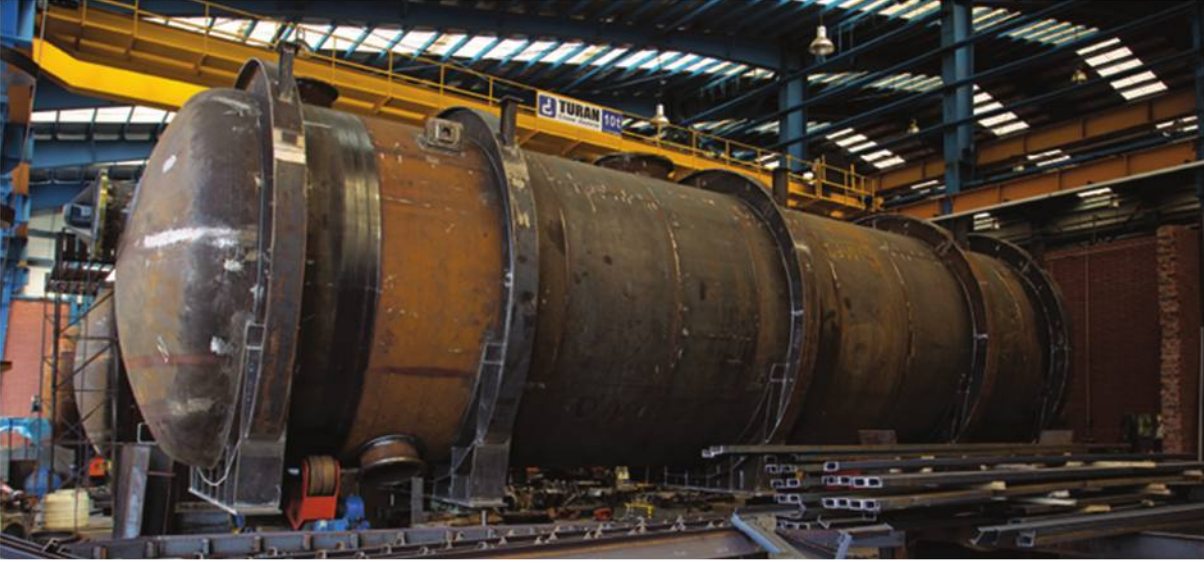
● The sand filter of desalination of Bandar Abbas
